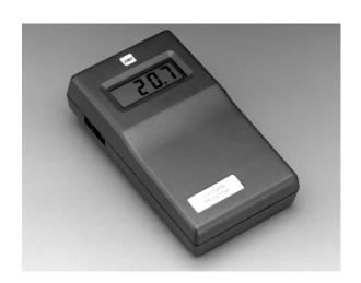
The Model 55 is a self-contained, lightweight, battery operated personal oxygen deficiency monitor. This easy to use monitor does not require any adjustments by the user other than routine calibration. The monitor reads true percent oxygen in the presence of any diluent including humidity and will not be affected by barometric pressure changes caused by elevation or weather changes.
